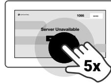
Touch the touchscreen **5 times very quickly** to enter **the service menu**. A window for entering the PIN code will appear. The PIN code is **"1066"**.
