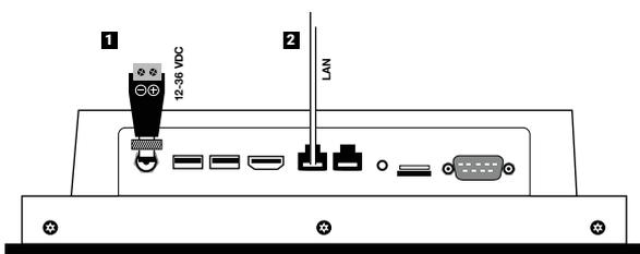
**2** Connect the Ethernet cable to the ETH 1 port.
