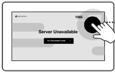
Touch the panel in **the upper right corner on Service PIN** and enter the PIN code **"1066"**.
